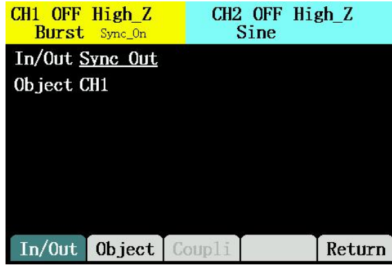
Figure 2-36 multiplex port interface output setting
