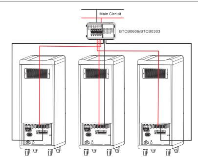
Step 1: The schematic diagram of the parallel connection of three battery packs is shown in Figure 1.
