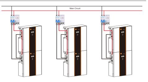
**Step 3**: The schematic diagram of the parallel connection of six battery packs is shown in Figure 3.
