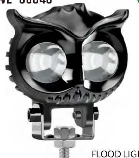
FLOOD LIGHT SHAPE 9-50V DC | 13W+13W | Yellow+White | IP67 | 67.5x72.5mm
