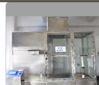
Saline Spray Testing
