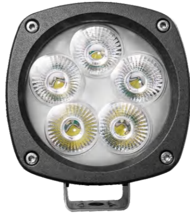
FLOOD + SPOT LIGHT SHAPE 9-36V DC | 50W | IP68 | 108 x 109 x 81 mm
