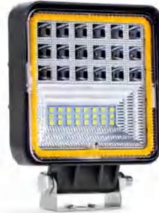
FLOOD + SPOT LIGHT + ORANGE CLEARANCE LAMP 9-36V DC | 45 W | IP67 | 110 x 110 x 35 mm
