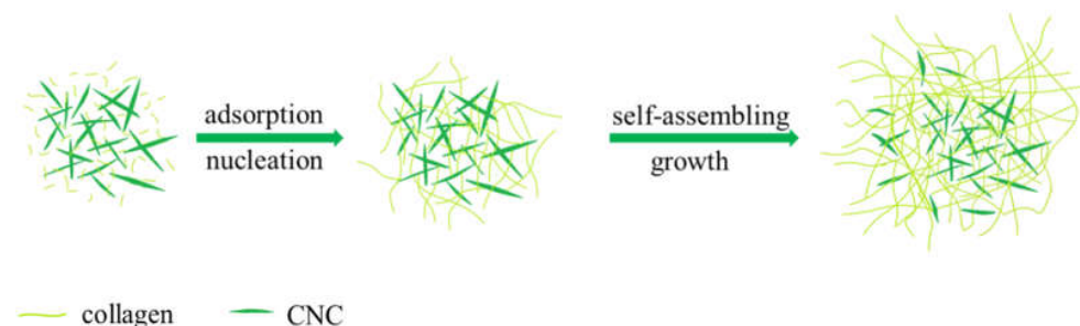
Scheme 1. Schematic illustration of the collagen self-assembly in the presence of CNC.
