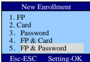
Input a user ID and click “ok”. Press a finger 2 times. If both pressing are ok, input the same password 2 times. Now the
