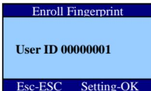
In the fingerprint enrollment screen, press fingerprint 2 times. If both image are near, the enrollment succeed.
