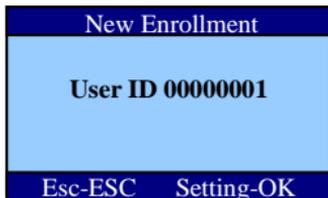
Swipe a card in the card sensing area. In the fingerprint enrollment screen, use a finger to press 2 times. If both pressing are ok, the enrollment is succeeded.
