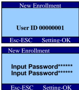
Note: In the verification, press fingerprint and you will be prompted to input the password. If password is correct, the verification is ok.
