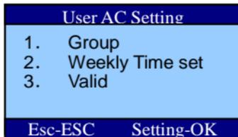
If the user do verification, the fingerprint/card machine will determine the group of the user and see whether it has rights of opening door. If the verification time is within the allowed time zone of the group, the door will be opened. Otherwise, the door
