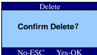
Press "ok" to confirm deletion or "esc" to abort the action.
