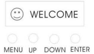
The Control Panel shows the current state of the unit. It is used to select the operating mode, as well as the sub-features. For a detailed layout of the control panel functions, please see the "menu map" section on the following page.
