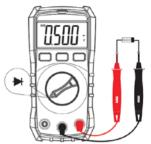
normal structure of silicon semiconductor, the forward voltage drop should be  $0.5V \sim 0.8V$ . If you mistake the test leads connection, it will display "OL" and means it is an open circuit. Now the black test lead connect to the "+", and the red one to "-".
