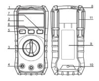
6-1. Sound alert indicator6-2. LCD display6-3. Function / range knob
