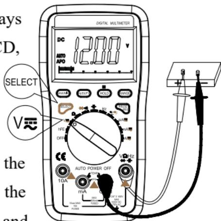
3. Connect the test lead to the tested circuit in parallel, the polarity of the red test lead and the tested voltage value will be displayed on LCD simultaneously.
