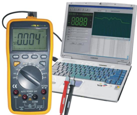
2. Auto Power Off Stop working for 15 seconds, the instrument will auto power off, and get into the sleeping mode. The buzzer inside will sound 5 times one minute before powering off, there is a long sound one minute later and the instrument gets into the sleeping mode. Press any key to restart the power.
