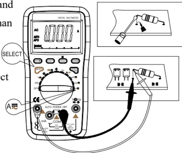
parallel when the test lead is inserted in the current input terminal, otherwise it is possible to damage the instrument or endanger the safety of the users. Cut the connection between the test lead and tested circuit at once after measurement.
