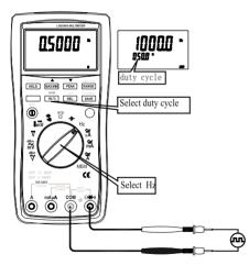
Figure 3-12. Frequency and Duty Cycle Measurement
