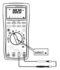
Figure 3-8 Continuity Test Measuring Capacitance (See Figure 3-9)
