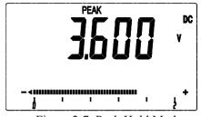
Figure 2-7. Peak Hold Mode Using MAX MIN Mode
