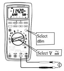
Figure 3-2. dBm Measurement Note If dBm is displayed, check that the reference resistance value closely matches the impedance of the system being measured.
