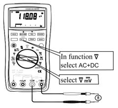
Figure 3-3. DC Volatage Measurement
