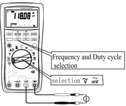
Figure 3-1. AC Voltage Measurement
