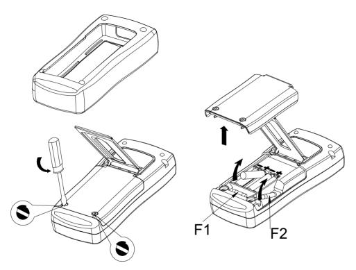
Figure 6-1. Battery and Fuse Replacement
