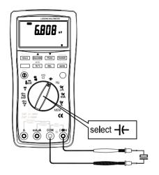
Figure 3-9. Capacitance Measurement Select
