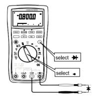
Figure 3-7. Diode Test Select₩; select Note
