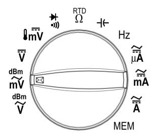
Figure 2-3. Rotary Switch
