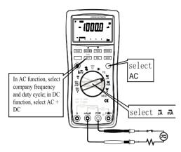
Figure 3-10. Current Measurement
