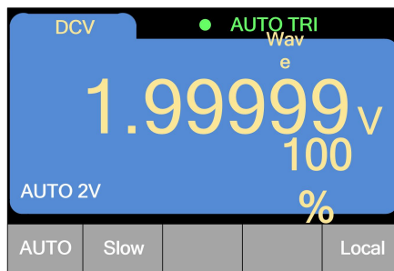
Figure 2.8.5 Switch from the interface of square wave output to that after the measurement of DC voltage
