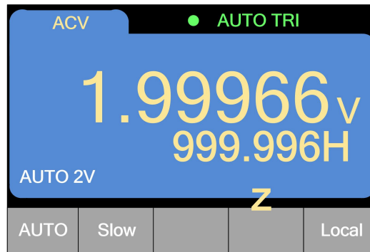
Figure 2.1.3 AC Voltage Measurement
