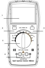
(5). Measuring switch: Press the key to start measure .
