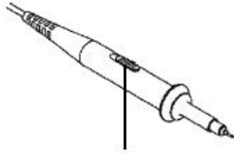
Figure 0-4: Probe Attenuation Switch
