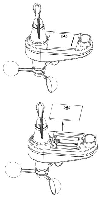
3. Inserting 4xAAA batteries in the battery compartment, and close the battery door.
