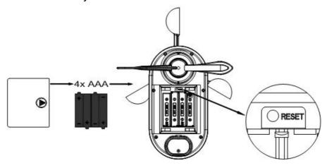
4. The wind sensor LED indicator will light for 4 seconds, and then flash once per 16 seconds thereafter. Each time it flashes, the sensor is transmitting data.
