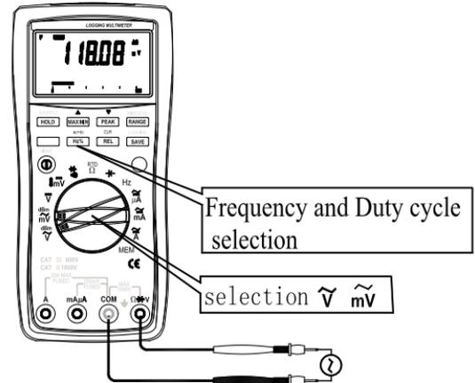
Figure 3-1. AC Voltage Measurement
