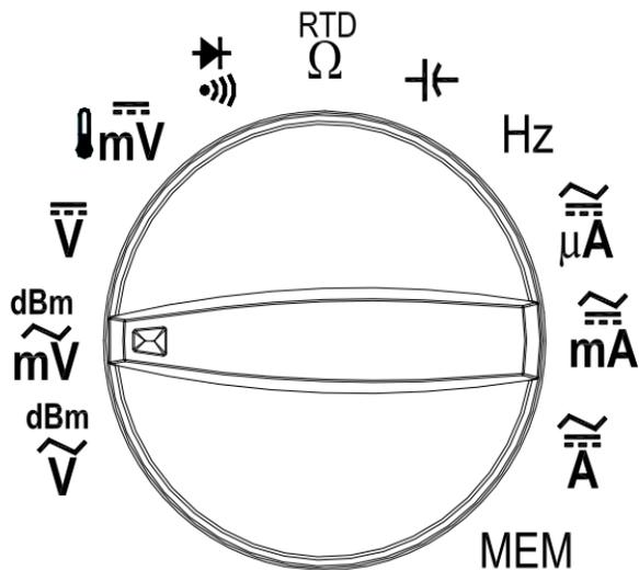
Figure 2-3. Rotary Switch
