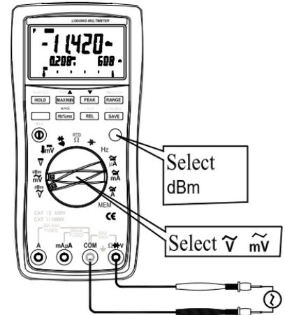
Figure 3-2. dBm Measurement
