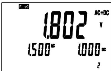
Figure 2-12. AC+DC Measuring Mode
