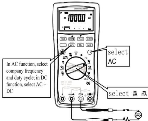
Figure 3-10. Current Measurement
