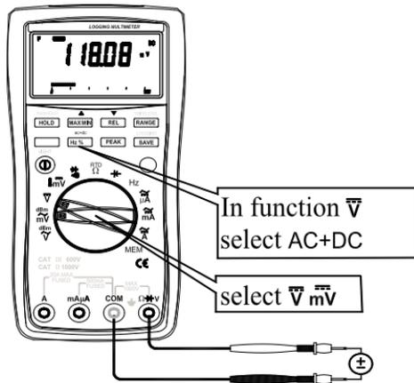
Figure 3-3. DC Voltage Measurement
