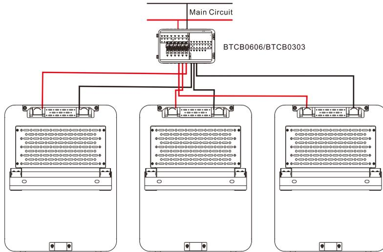
**Step :** The schematic diagram of the parallel connection of three battery packs is shown in Figure 1.
