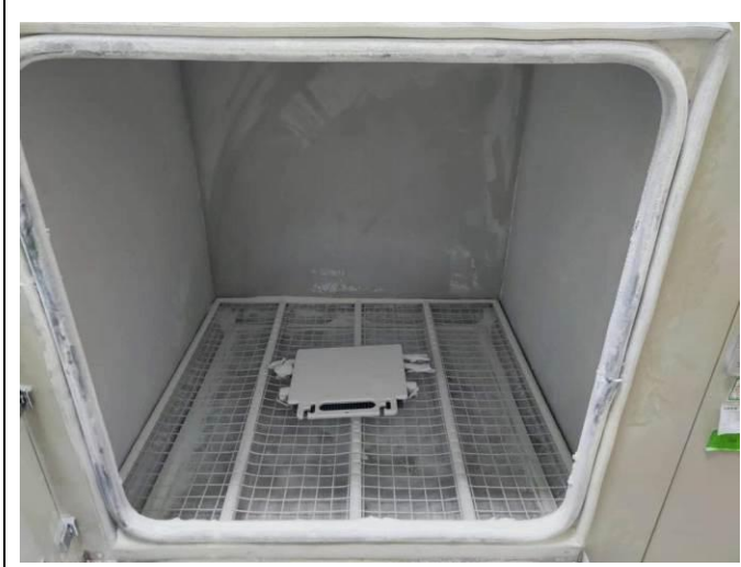
Photo 3 After the dust-proof test
