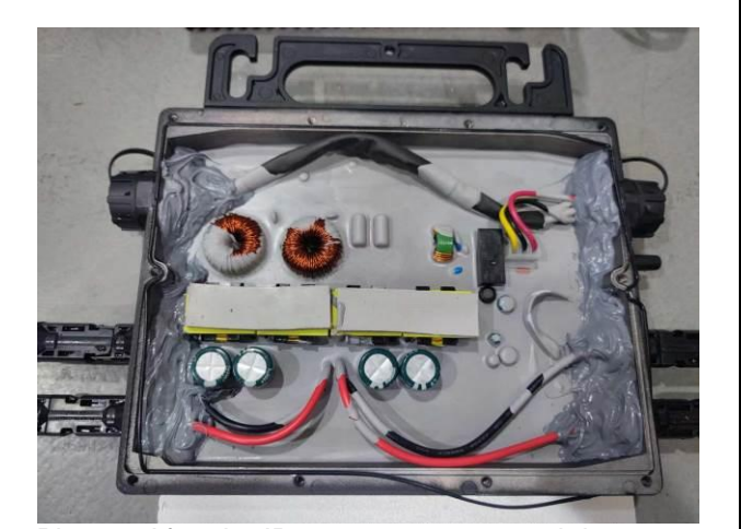
Photo 6 After the IP67 test, no water and dust entry into internal.
