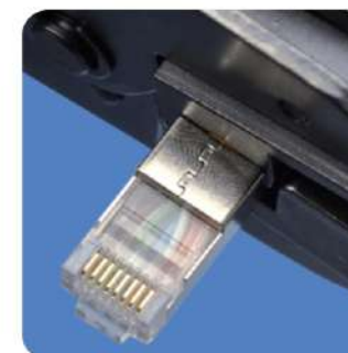
10.Put the tail part into crimping tool and press
