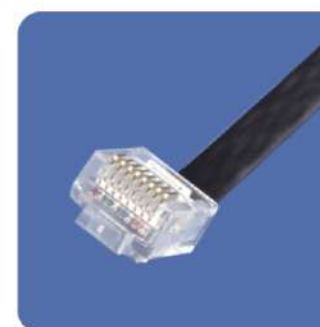
5.Check the wires' position.
