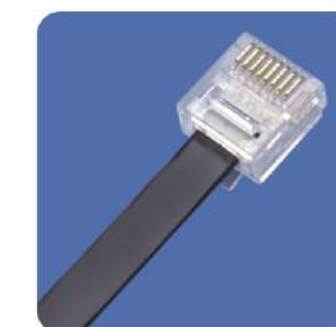
4.Put the wires into the end of plug.
