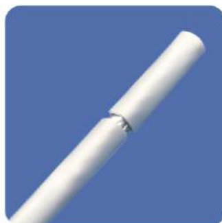
2.Strip the insulation outer sheath of the network cable, about 15mm.
