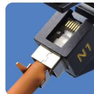
9.Put plug into crimping tool and press
