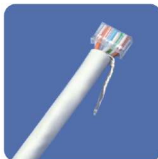
4.Thread the core wires into the core plug. (White Orange/Orange/White Green/Blue/White Blue/Green/White Brown/Brown)
