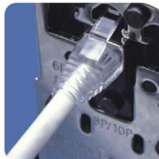
7.Place the RJ45 plug into a hand tool crimping die for compression.
