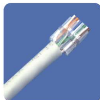
6.Thread the core wires into the core plug: (White Orange/Orange/White Green/Blue/White Blue/ Green/White Brown/Brown)
