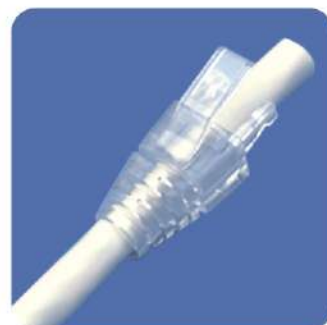
1.Thread the boot into the network cable.
