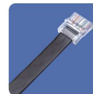
3.Click the insert and cut extra wires.
