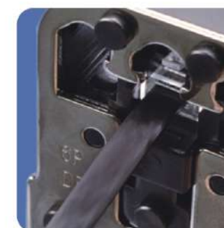
6.Insert the cable to crimping tool.
