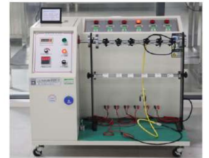
Wire Bending Tester Function: Tests the flexural strength of wire materials.
