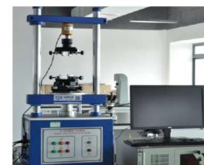
Servo Inserting machine Function: Detection of insertion force and pulling force.
