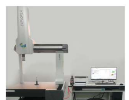
HEXAGON Explorer Classic Function: Hexagon three-coordinates measuring machine
