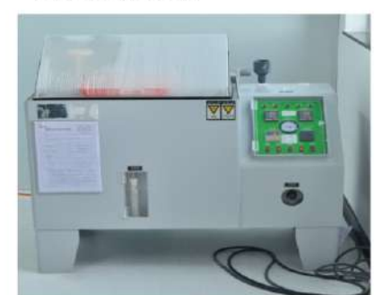
Salt-Fog Spray Tester Function: Ensure the plating of gold sheet and shielding shell products qualified.
