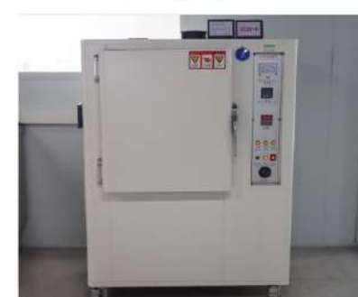
Yellowing Resistance Tester Function: Tests the aging and yellowing resistance performance.
