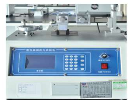
Insertion & Withdraw Tester Function: Test the RJ45 plug and pull endurance of RJ45 plug and RJ45 keystone jack seat.
