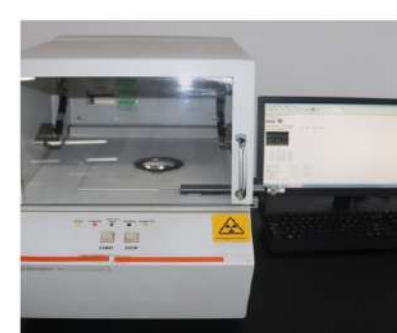
Film Thickness Tester Function: Check gold-plating thickness.
