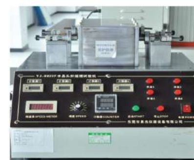
Shrapnel Bending Tester Function: Physical function detection, ensure the RJ45 plug shrapnel bending degree.
