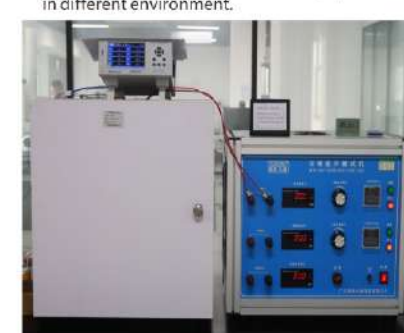
Dual-Channel Temperature Rise Tester Function: Detects the temperature increase at a specific point of the product.
