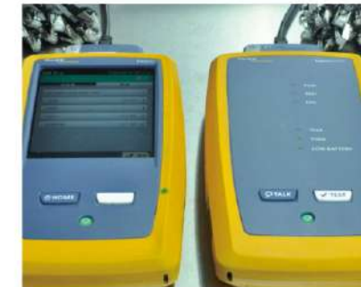
Fluke Tester Function: Ensure the matching performance of RJ45 plug and patch cord qualified.
